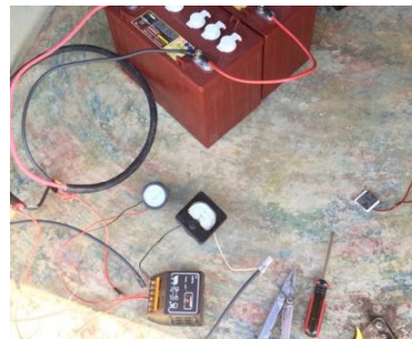
Fig. 9: The optimal tilt measuring apparatus set up by the students at the ITCS. With analog current and voltage meters, the power output at various panel tilts could be assessed in real time. This allowed the students the chance to develop a physical relationship with the concept of panel direction.
