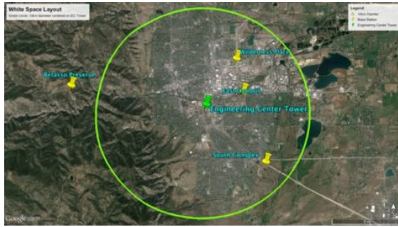
Figure 4: A map of the Boulder, Colorado showing the locations of the 3 local client stations (Wilderness Place, East Campus (SPSC) and South Complex) all within 5km of the Engineering Center (EC) Tower, a range represented by the green radius. The Betasso Preserve location is intended for mobile unit testing.
